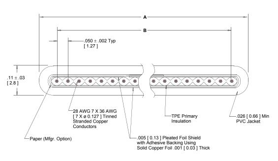
Note: Blue marking on one edge of primary cable designates wire #1.
